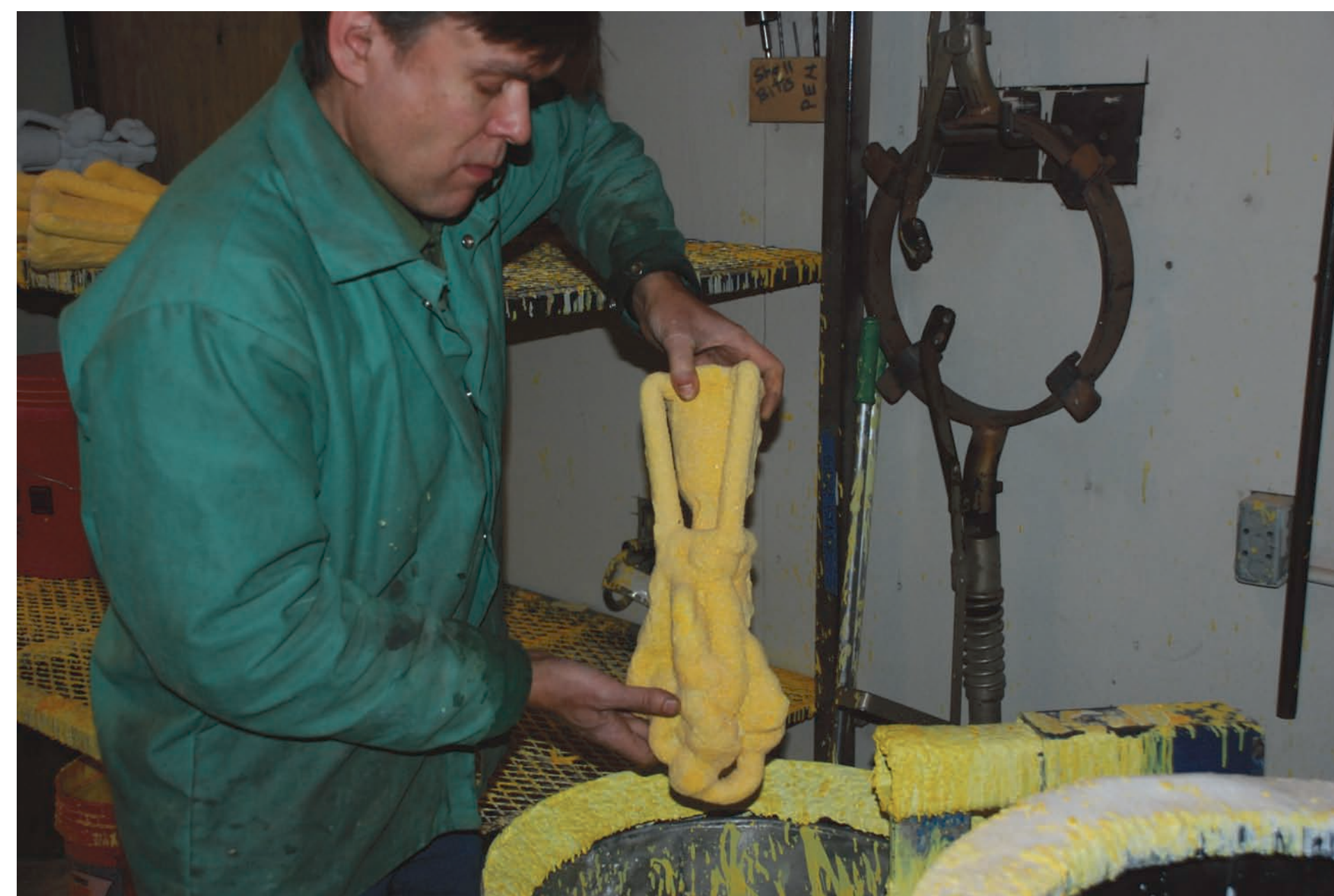
Don Myhre dipping the figure into the colloidal silica shell bath
