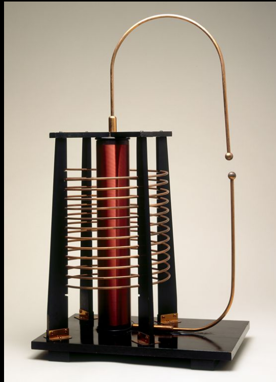
98.276.180 DATS Nikola Tesla, Welch Scientific Company, "Tesla Coil" high-frequency discharge demonstrator, 1931 Steel, copper, wire, wood 29 x 18 1/2 x 12 1/2in. (73.7 x 47 x 31.8cm)
