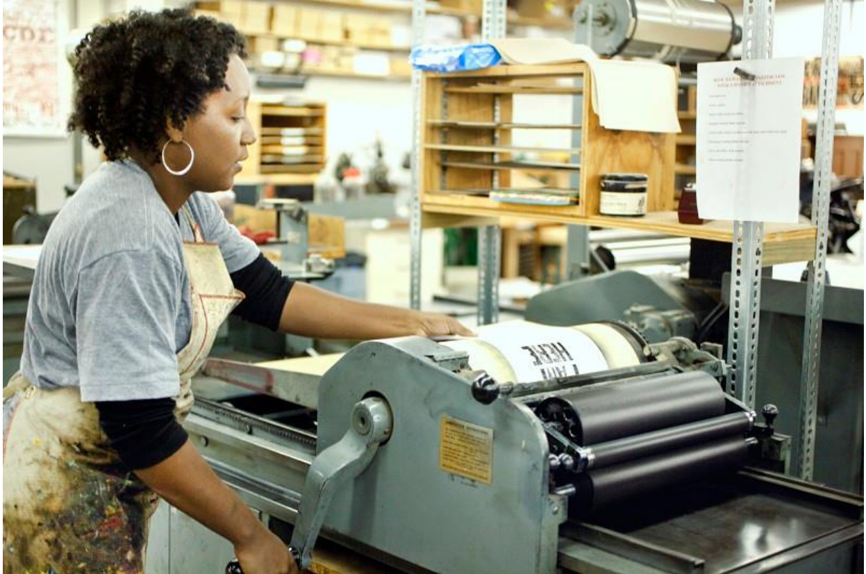
Cranking it out: Delita turns up the creative heat and demonstrates letter press printing on a Vandercook Letter Press.
